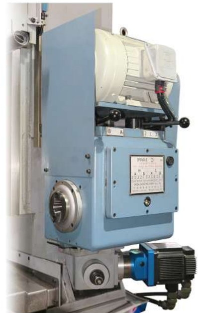
H 齒輪頭構造(主軸不可伸縮) H Gear Type Spindle (Six-Steps Gearbox)
